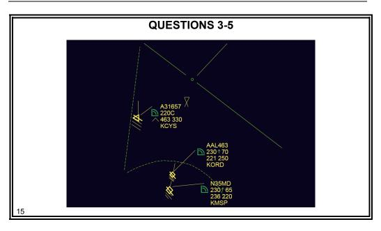
3. AAL463 and N35MD are being handed off to an ARTCC from approach control. The distance between these two aircraft is **only** 3½ miles. Is this less than minimum separation? Explain your answer.
